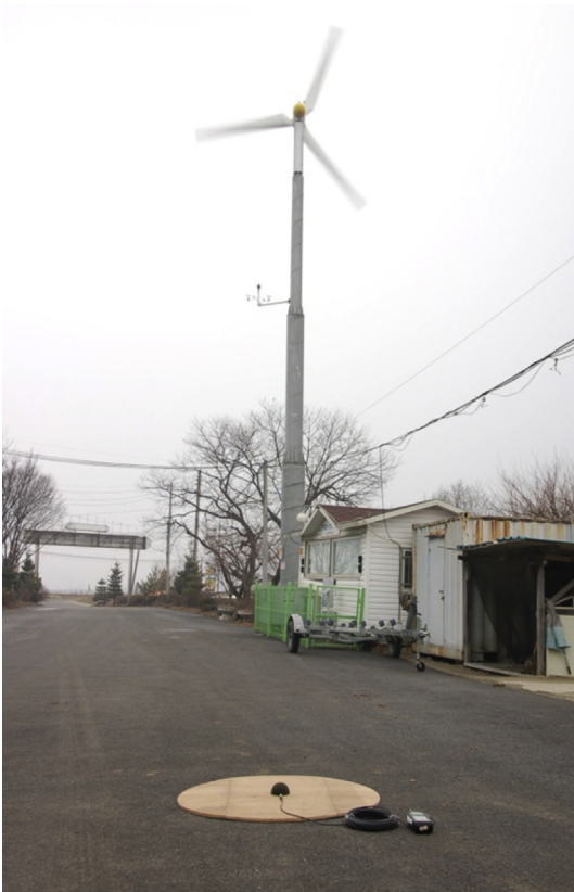
Fig. 8. Configuration of the 10 kW class noise measurement test.
